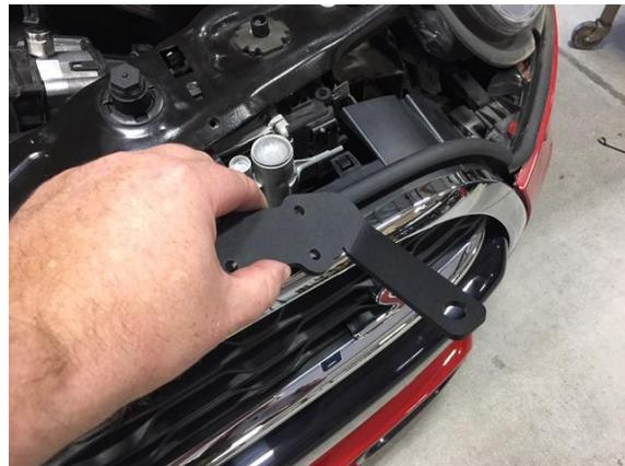
Here's the opening that the bracket will protrude through once installed:
