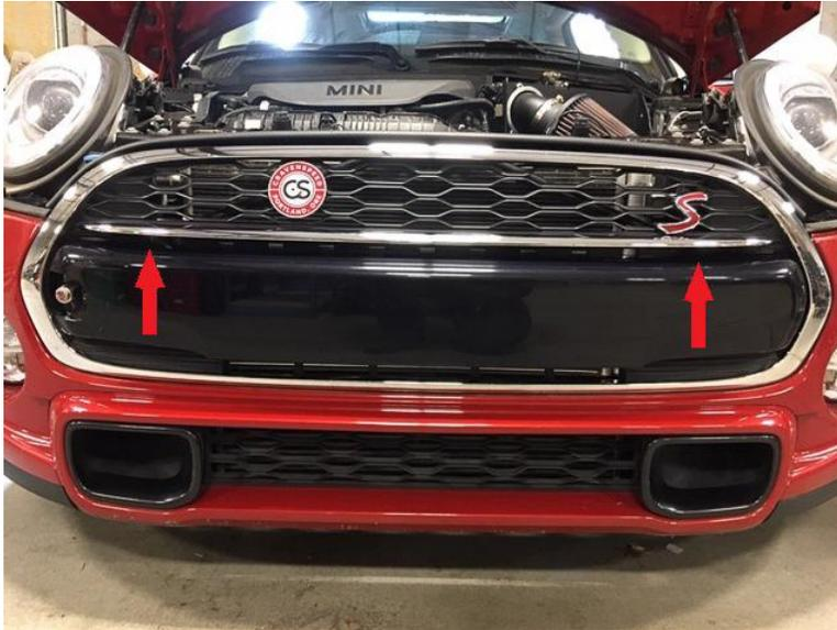
5. Grab a bracket in hand and enter behind the grill, placing the light mounting tab through the slot below the grill. The four-holed mounting portion of the bracket should lie flat against the v-brace core support bar.
