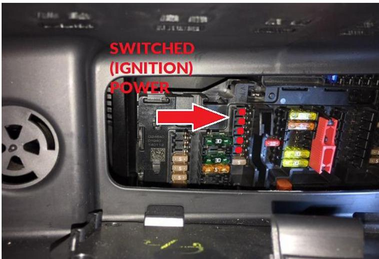
10. Feed your white wire up and through the opening in the back of the glove box and utilizing your crimp tool, fasten the 'Add-a-Circuit' to the end of the wire. Place the 1mA mini fuse into the top section of the 'Add-a-Circuit' and then plug it into one of the designated switched (ignition) power sources.
