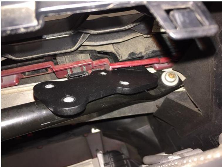
6. Insert the 1/4-20 x 1.25" stainless cap screws through the bar mounting portion of the light brackets with the cap heads facing up. Place the 'dog bone' shaped clamp on the backside and tighten the cap screws evenly with your 3/16" hex key wrench. Ensure that the light mounting tabs that come through the slots under the grill are level before performing a final tightening. Hand-tight is fine.. do not crush or deform the core support bars.
