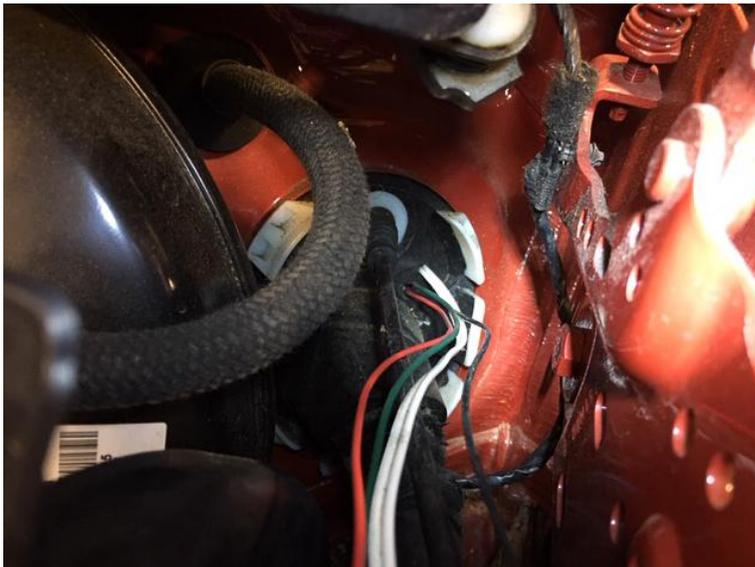
6. Open your driver side door and use a trim panel tool to pop off the side dash panel. Shine a light inside and back towards the hole you drilled through the firewall plug, locate the PIAA wires and pull them through. Resolder the two wires back together and heat shrink/wrap them.
