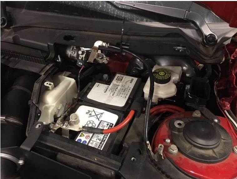
3. We won't need to remove the entire grill for this install, but we do need to loosen some stuff up to make room to work. Remove the 5 T30 torx screws across the top of the grill and you should be able to flex the grill forward just enough so that you can access the v-brace support bars behind it.
