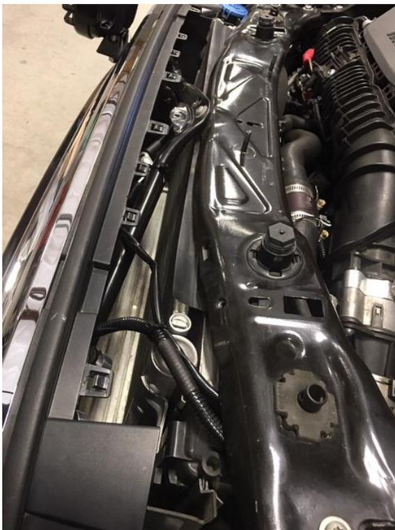
2. Next, we need to locate a suitable location for the PIAA light harness relay. It will need to be mounted vertically so that water cannot collect inside of it, and the driver side headlight has a mounting point that will fit the bill nicely. Remove the 10mm screw from the headlight mount and pull off the clip-nut with a set of pliers. Replace the 10mm screw and affix the relay to the inboard side using the supplied M6 locknut and flat washer.
