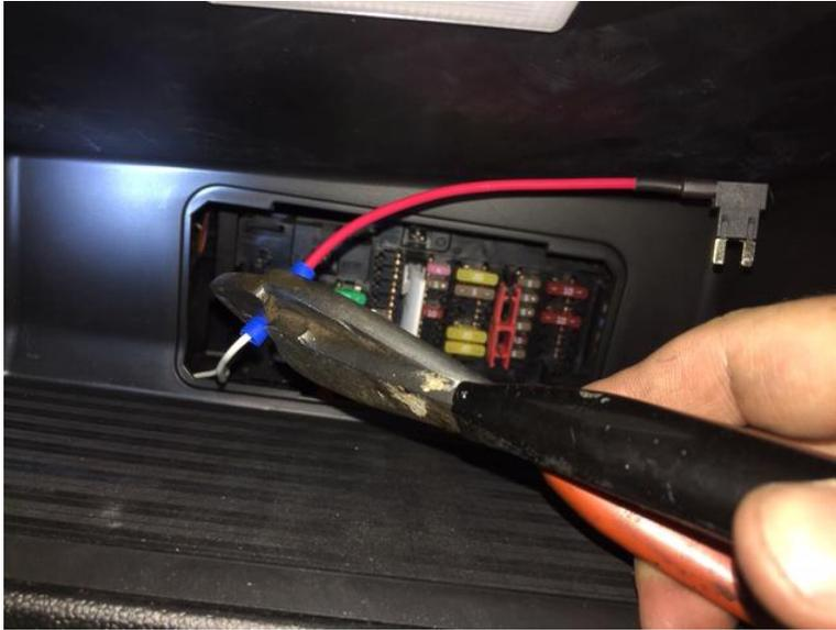
11. Loop any excess wiring together and secure it under the dash with a couple zipties.
