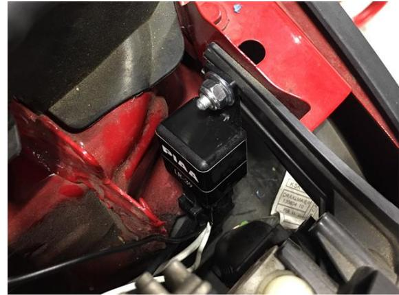
3. Coil up any excess wiring between the relay and the lights and zip tie it out of the way. With your 13mm socket and ratchet, connect the relay ground to the battery ground bolt attached to the body of the vehicle and the relay power to the accessory post on the positive battery terminal.
